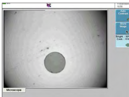
Connector image display on the T-BERD/MTS optical test platforms
